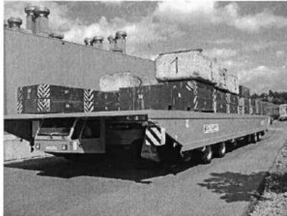
Photo shows a 650 ton ship section and engine transporter during load test
